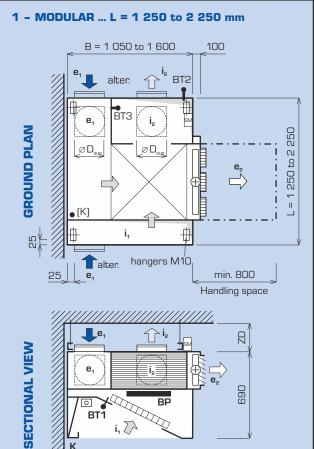
Figures show the DiNER-TN hood delivered in the right-hand design as standard. When requested, the mirror (left-hand) design can be delivered, including heating water distribution.
