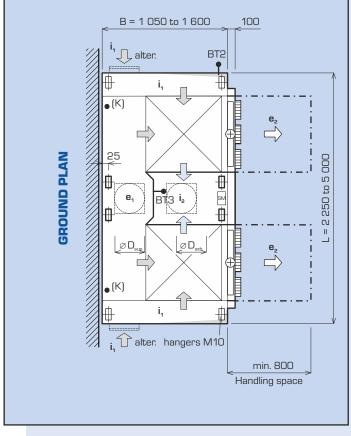
HEATING WATER DISTRIBUTION AND CONNECTION BT2 ⊕ **GROUND PLAN** ₩ e, ⊕ Standard locations of the central heating (UT) are shown, different location is possible upon request
